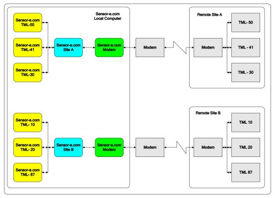
Figure 2-4: Instruments, Sites, and Connectors
