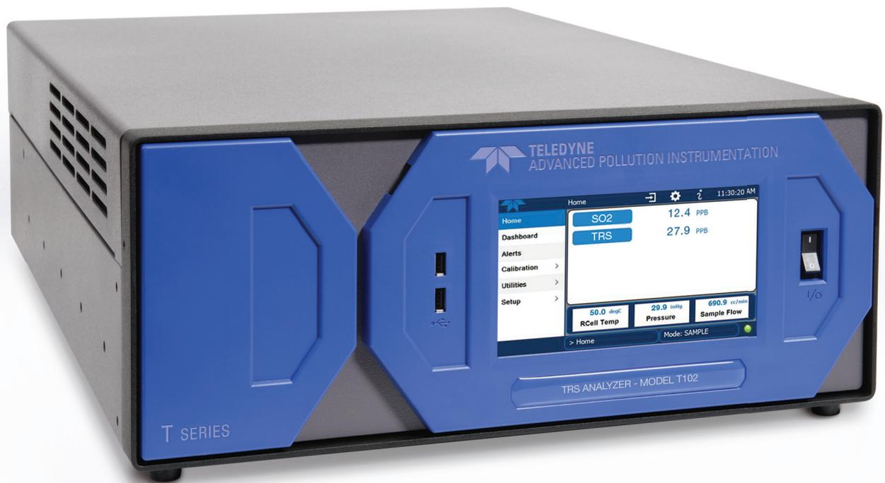
The Model T102 TRS analyzer uses the proven UV fluorescence principle to measure Total Reduced Sulfur at levels commonly required for ambient air monitoring.
