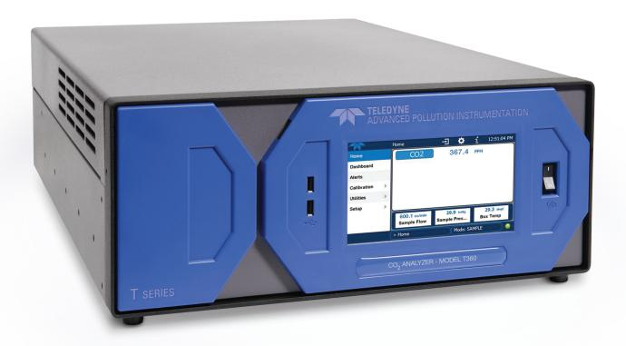
Using a gas filter correlation wheel, the Model T360  $\rm CO_2$  analyzer measures carbon dioxide by comparing infrared energy absorbed by a sample to that absorbed by a reference gas according to the Beer-Lambert law.
