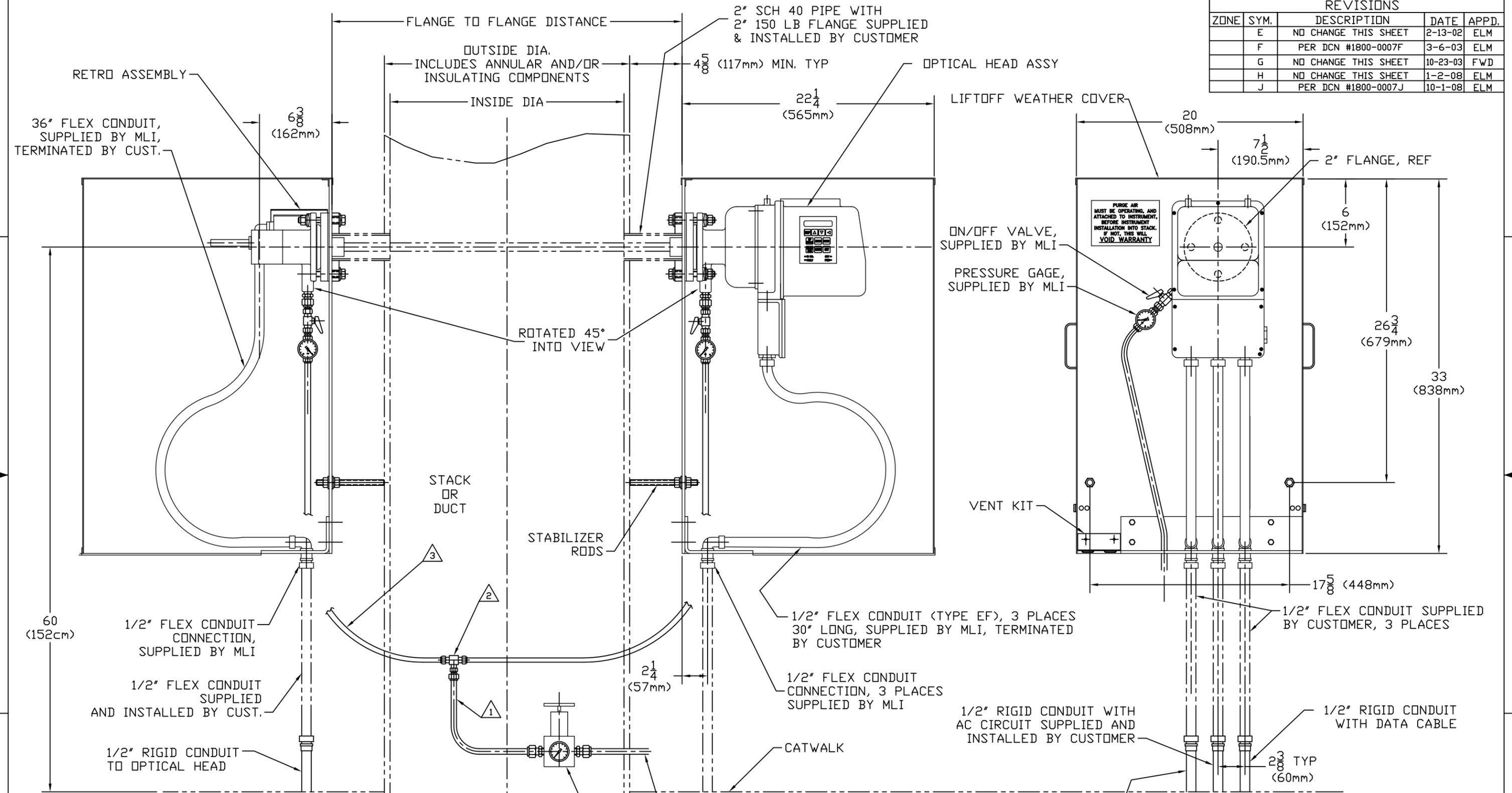
1 CUSTOMER TO SUPPLY AND INSTALL 1/2"OD x 3/8"ID x 6 FT LONG TUBE TO CARRY INSTRUMENT AIR FROM THE REGULATOR TO THE TEE. PLANT AIR SYSTEM TO SUPPLY A TOTAL FLOW OF 25 CFM MINIMUM AT A DYNAMIC PRESSURE OF 30PSI OR HIGHER @ THE REGULATOR. PRESSURE AT THE ON/OFF VALVES SHOULD BE THE SAME AS THE REGULATOR PRESSURE WITH THE VALVES CLOSED. PLANT PRESSURE MAY NEED TO BE HIGHER IF THERE ARE RESTRICTIONS UPSTREAM IN THE PLANT AIR SYSTEM. THE REGULATOR SHOULD BE RATED FOR HIGH FLOW.
