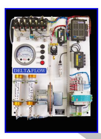
The DELTAFLOW, Model DF180, is a state of the art differential pressure measurement system used to calculate gas velocity and pollutant mass emissions in square, rectangular or circular air ducts and stacks using either single or multi point measurements. It especially excels in gas streams with challenging properties such as high temperature, moisture content, pressure, particulate loading and corrosive.
