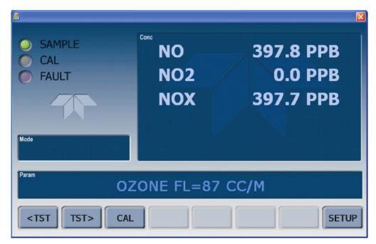
Figure 3-2: Display Screen and Touch Control
