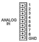
Figure 3-7: Analog In Connector
