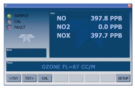
Figure 4-1: Front Panel Display
