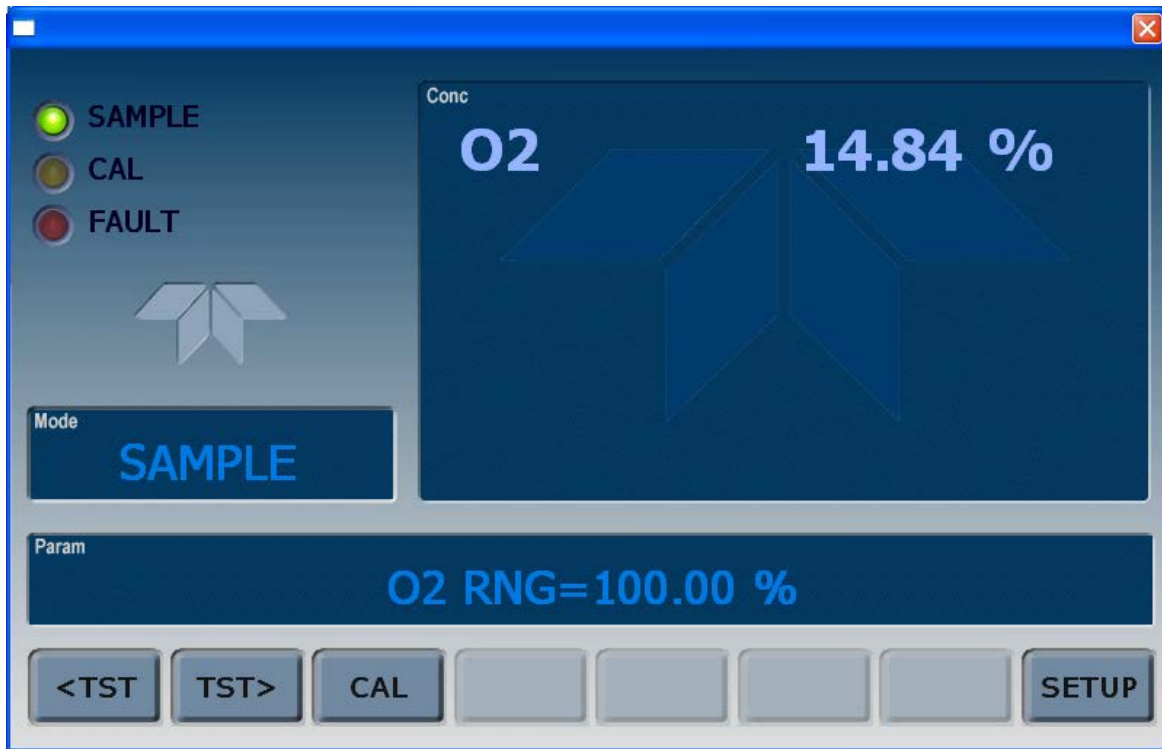
Figure 3-2. Display Screen and Touch Control
