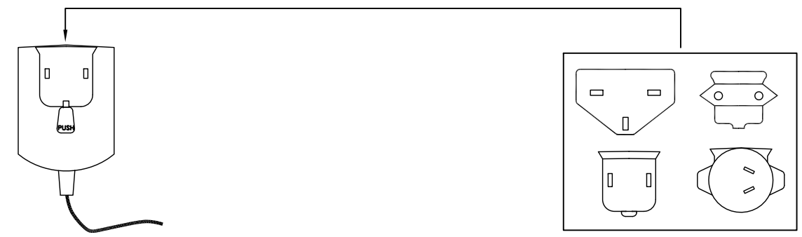
523887 UNIVERSAL AC PLUG KIT, SLIDE PLUG FOR DESIRED SERVICE ONTO 1903-2040-01 SUPPLY AT LEFT.
